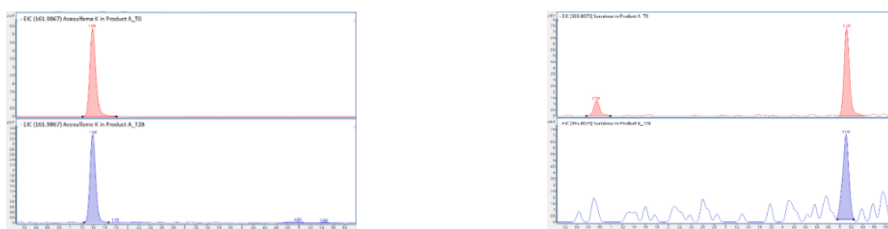
Figure 1. Acesulfame K. Extract ion chromatogram at the beginning (T0) and at the end (T28) of the RBT. Figure 2. Sucralose. Extract ion chromatogram at the beginning (T0) and at the end (T28) of the RBT.
